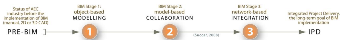
Fig. 7. BIM maturity is subdivided into three stages – linear view
